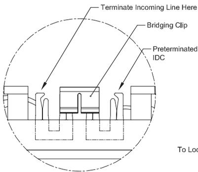
If using ICC's bridging clips use the configuration shown above.
